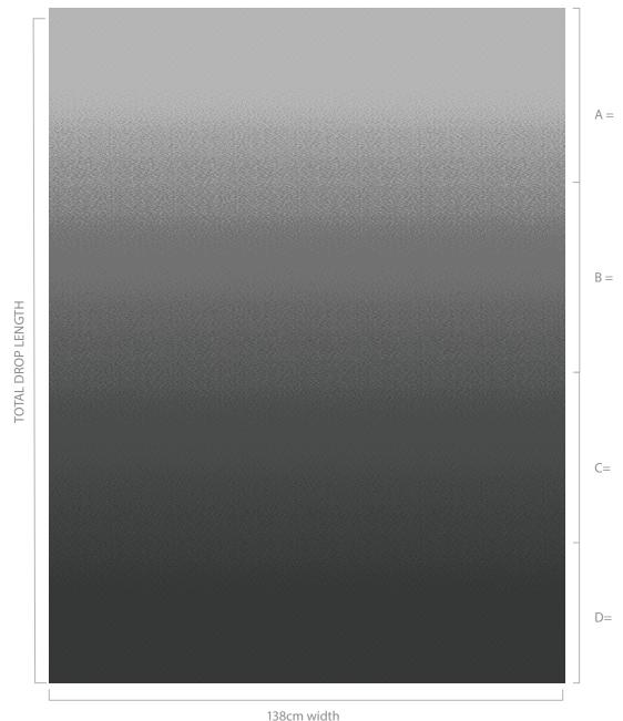
SECTIONS A, B, C & D MUST BE NO LESS THAN 32CM EACH
